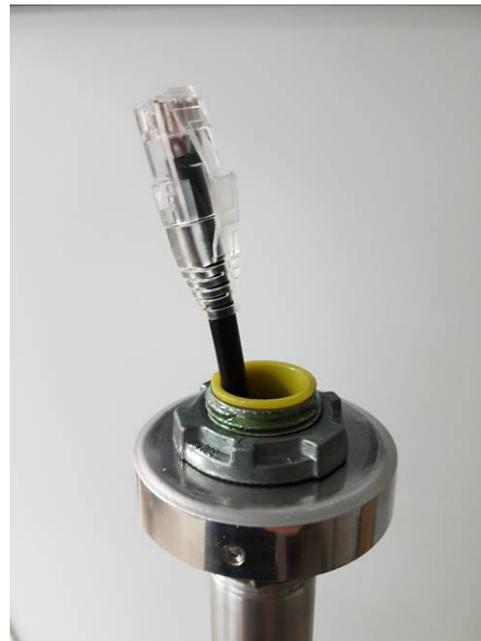
Insert the cable connector into the RJ45 connector on the ANT-2.
