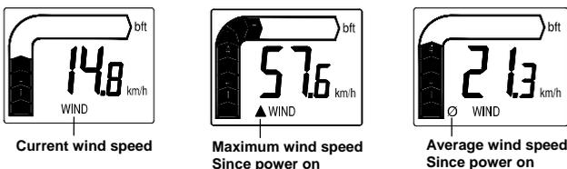
To toggle between current wind speed, maximum wind speed and average wind speed, simply press the "+" key:
