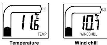
By pressing the "+" key the display will toggle between temperature and wind chill. When the temperature is outside the range from -29.9°C to +59°C, there will be no wind chill measurement.
