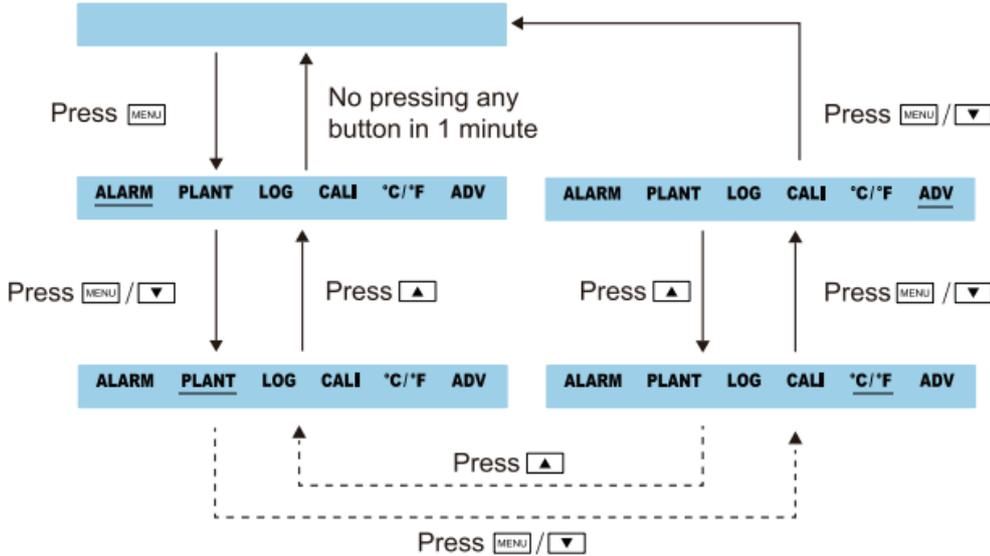
To select the function, press Enter when it is underlined by the flashing bar. Note that after one minute if nothing is pressed, the Main Menu will disappear, and the device will revert to the normal state.
