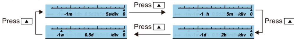
The table below shows the available Zoom Levels for all parameters CO2/ Humidity/ Temp.as well as the duration of each division for corresponding Zoom Levels:
