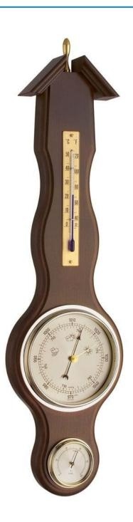
Banjo barometers have been around since the mid 1800s, and are still the most popular design. The central dial shows the barometric pressure information, the top part is a temperature scale, and the bottom is a humidity dial. This TFA Dostmann barometer is German-made, and is of a beautiful quality.
