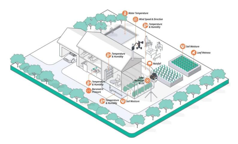
Sensor Transmitters are the building blocks of your custom network of sensors. They can be positioned indoors or outdoors and are capable of transmitting data up to 1,000 ft. (300 m). Each transmitter can support up to five sensors, including an Anemometer, Rain Collector, Temperature Probe or Temperature & Humidity Sensor, UV Sensor and Solar Radiation Sensor.
